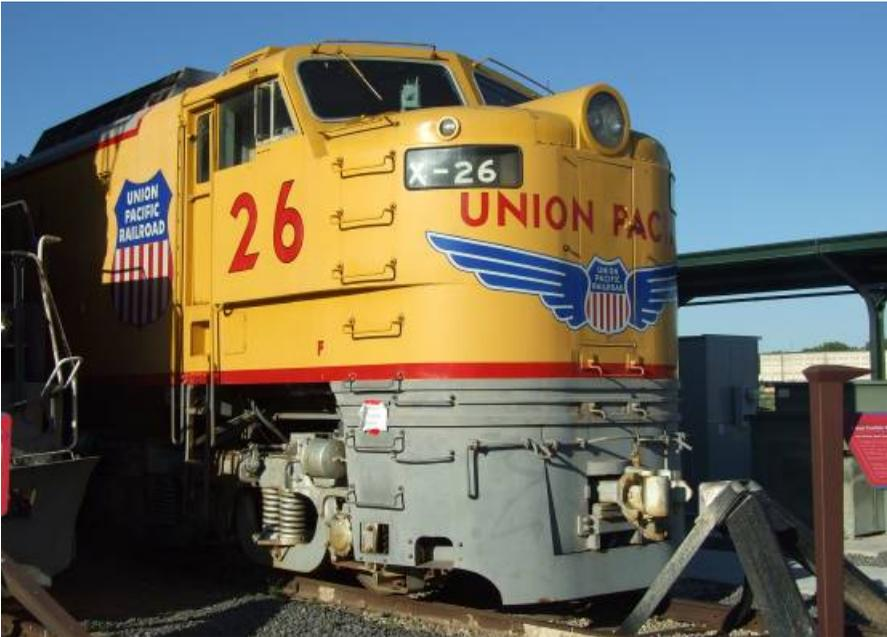
Above: Standard gauge “Big Blow” UP 26 on display at Ogden, Utah USA. The loco had an 850hp auxiliary diesel in the A unit shown above, an 8,500hp gas turbine in the B unit and a 91,000ltr fuel tender. It was capable of hauling 12,000t between Council Bluffs, Iowa and Ogden, Utah.
